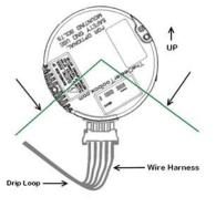
As installed in the air handler, the motor should be positioned with the connectors facing down between the 4 and 8 o-clock position, with the wiring harness formed into a drip loop.
